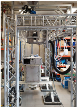
Photo of the sand test rig at SJJ with 60 kW sand cooler and 30KW IR emitter.
